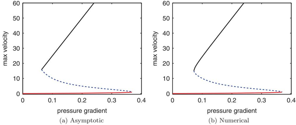
FIG. 16. (Color online) Plots of maximum velocity vs pressure gradient for  $\epsilon = 5 \times 10^{-4}$ . (a) Asymptotic solution. (b) Numerical solution of the boundary value problem.
