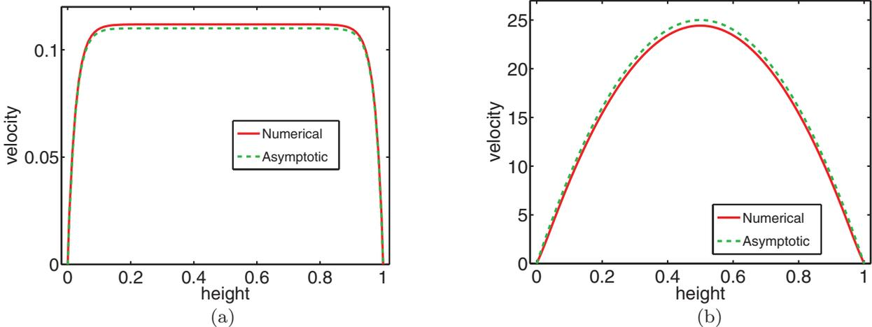
FIG. 13. (Color online) Comparison of the numerical solution to Eq. (12) and the asymptotic solution (a) on the lower branch in the plug flow regime and (b) on the upper branch in the parabolic flow regime for  $f = 0.1$  and  $\epsilon = 5 \times 10^{-4}$ . The error in the asymptotic approximation is around 2% in both cases.
