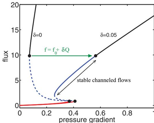
FIG. 10. (Color online) Flux vs applied pressure gradient for  $\epsilon = 5 \times 10^{-4}$  for  $\delta = 0$  and  $\delta = 0.05$ . The curve for nonzero values of  $\delta$  can be obtained from the curve for  $\delta = 0$ . As  $\delta$  increases more channeled solutions become stable and the range of pressure gradients where there are multiple solutions decreases.
