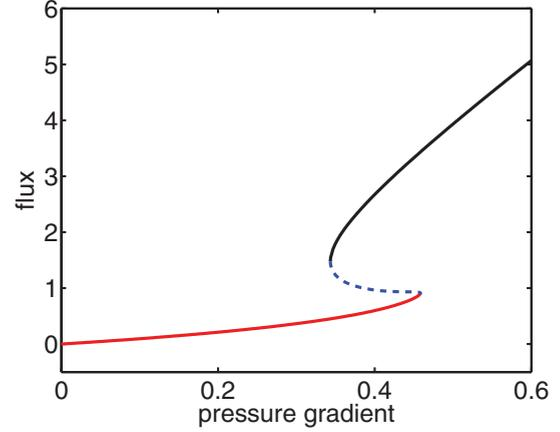
FIG. 8. (Color online) Flux as a function of applied pressure gradient, where the velocity profile satisfies Eq. (17) which includes the effect of pressure relief. The value of  $\epsilon$  is  $5 \times 10^{-4}$  and the value of  $\delta$  is 0.1. The unstable solution is represented by a dashed line.
