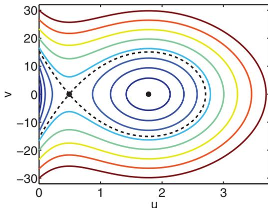
FIG. 14. (Color online) Level sets (not equally spaced) of the energy function (29) which correspond to solutions of the system (26) and (27). The two equilibrium points are marked with dots. The stable and unstable manifolds of the smaller equilibrium point are plotted by the dashed curve. There is a homoclinic orbit which encircles the larger equilibrium point. The parameters are  $f = 0.30$  and  $\epsilon = 5 \times 10^{-4}$ .
