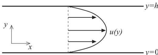
FIG. 4. To investigate channeling we consider the flow between two infinitely long parallel plates located at  $y = 0$  and  $y = h$  driven by an applied pressure gradient. The flow is unidirectional and the flow profile  $u(y)$  is a function of only the height between the two plates.
