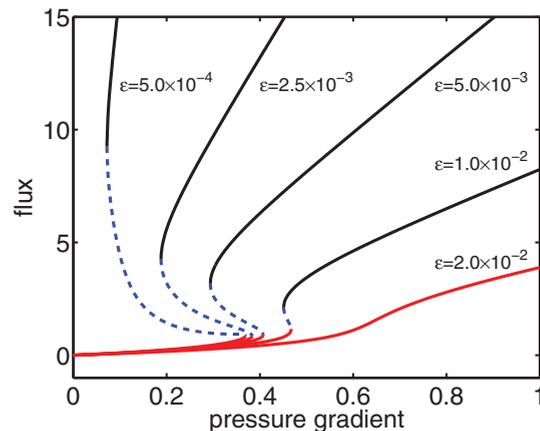
FIG. 11. (Color online) Flux vs pressure gradient for different values of  $\epsilon$  with  $\delta = 0$ . For large enough  $\epsilon$  there are no channeled solutions.
