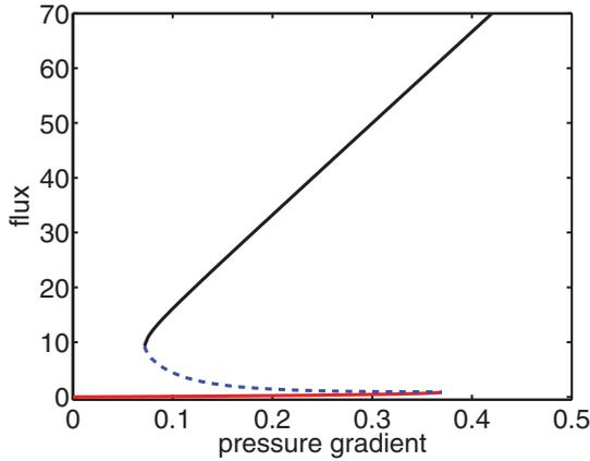
FIG. 5. (Color online) Flux as a function of applied pressure gradient where the velocity profile satisfies Eq. (12). The value of  $\epsilon$  is  $5 \times 10^{-4}$ . The unstable solution is represented by a dashed line.
