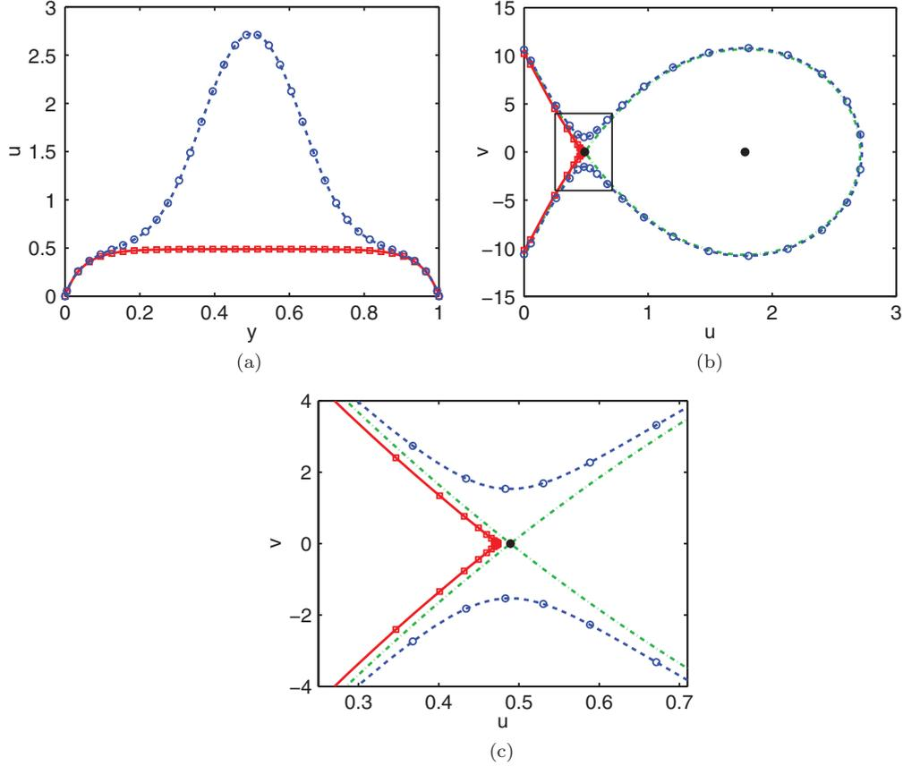
FIG. 15. (Color online) (a) Plug flow solution (red squares) and channeled solution (blue circles) for  $f = 0.30$  and  $\epsilon = 10^{-3}$ . (b) Solutions plotted in the phase plane along with the equilibrium points and the stable and unstable manifolds of the saddle point (green dash-dot curve). (c) Closeup of the solutions around the saddle point.
